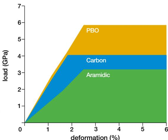
Structural fibres comparison: behaviour to monoaxial tensile strength
