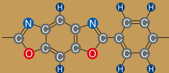
This synthesis polymer has a molecular structure able to establish strong chemical bonds with the special Ruredil X Mortar 750, and this plays a crucial role on the final performances of the new FRCM composite, P.B.O. + Ruredil X Mortar 750.
